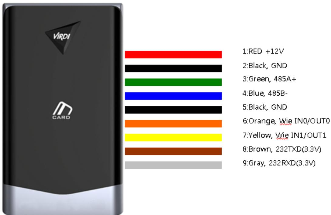
All readers require 4 wires for connection. All four wires should be home-run directly to the MCP040 controller.
