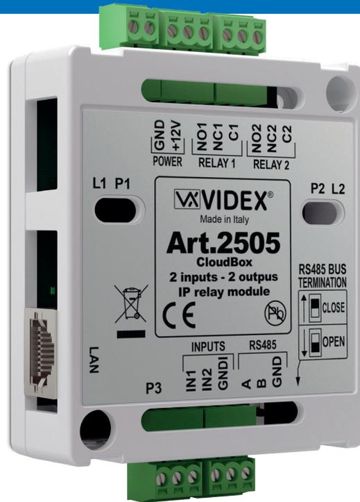
Art.2505 is an IP relay with two built-in relay and two active low inputs plus serial interface RS-485 for interfacing with other automation devices.
