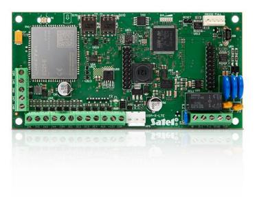
of INTEGRA Plus, the SMS content is based directly on the event log). It also enables remote programming of these control panels from a computer with the DLOADX program and administration of alarm systems using the **GUARDX** program.
