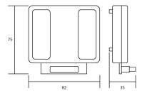
Wireless sounder interface module designed for use with modular wall sounders and sounder/VAD. When conventional sounder or sounder/VAD are fitted with this module they become fully compatible with all wireless translators and expander modules. EN54-18 and EN54-25.
